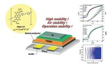
High-performance naphthalene diimide (NDI)-based conjugated polymer is developed as the active layer of n-channel organic field-effect transistors (OFETs). The solution-processable n-channel top gated OFET shows remarkably high electron charge-carrier mobility of up to 1.8 cm<sup>2</sup> V<sup>-1</sup> s<sup>-1</sup> with poly(methyl methacrylate) (PMMA) dielectrics.
