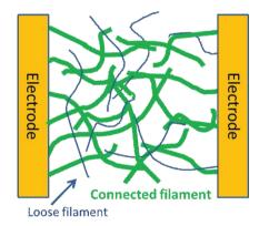
In-plane conductivity in PEDOT:PSS takes place via filaments. This conclusion is based on charge transport measurements that indicate quasi-one dimensional variable range hopping and is supported by transmission electron microscopy. At higher PEDOT to PSS ratios the number of connected filaments drastically increases, causing an orders of magnitude increase in conductivity, in good agreement with percolation theory.
