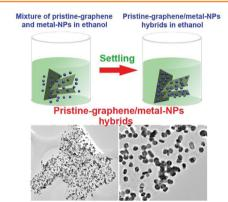
An environmentally friendly generic synthetic approach to large-scale pristine-graphene/metal-NPs hybrids via van der Waals interactions between the pristine-graphene and the metal-NPs is presented. Nanoparticles of different metals with various morphologies can be homogeneously attached on the defect-free pristine-graphene. The as-synthesized pristine-graphene/Ag-NPs hybrids show high surface-enhanced Raman scattering (SERS) sensitivity and can serve as ultrasensitive SERS substrates.
